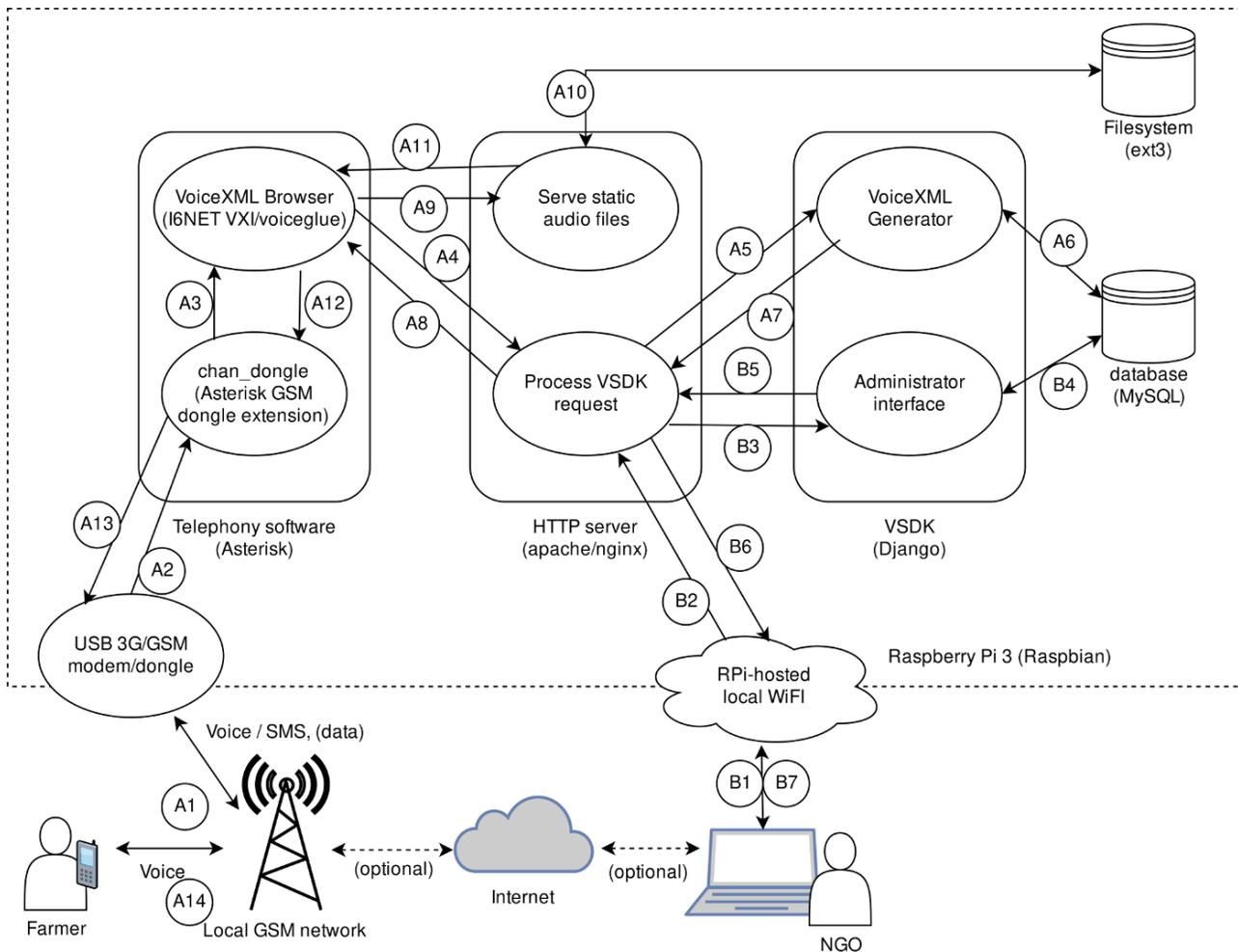
Figure 10: Overview of the KasaDaka system architecture
